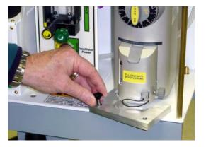
**B.** Remove the two holding knobs and spacer plate from the back plate located on the backside of the frame behind the vaporizer.
