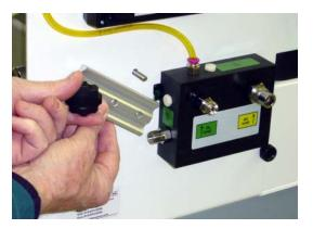
C. Pull the vaporizer forward and remove the inlet and outlet tubing connectors.
